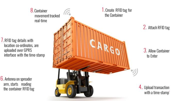
5. Unload container from trailer using container handling equipment
