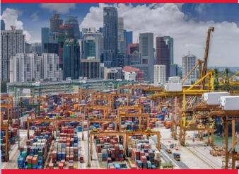
**Port of Singapore**, has installed RFID transponders into its container yard to create a multi-dimensional tracking grid. All of this helps them to track, manage the placement and location of their containers.
