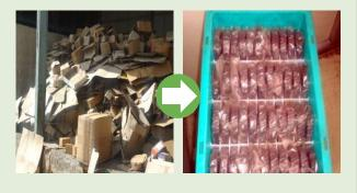
1,930 liters of diesel and 4.2 tons of  $CO_2$  was saved by using hydraulic press which compressed waste and helped vehicle take 8 tonnes of waste compared to just 2.25 tonnes earlier
