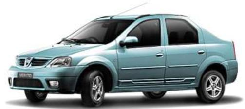
The Verito Electric is also India's first completely electric sedan and takes seven hours to charge fully and just an hour for a fast charge. On full charge, the electric Verito can travel 80 km and reach a top speed of 85 kph.
