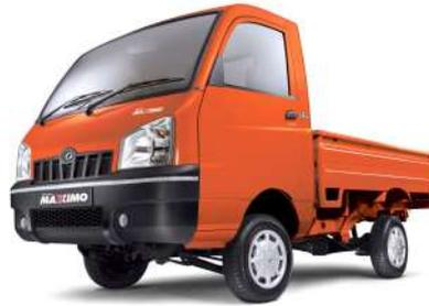
Maxximo EV has a range of 90 km and takes eight hours to charge the batteries of the passenger carrier. With a top-speed of 55 km/h, it has a maximum gradeability rating of 18%.
